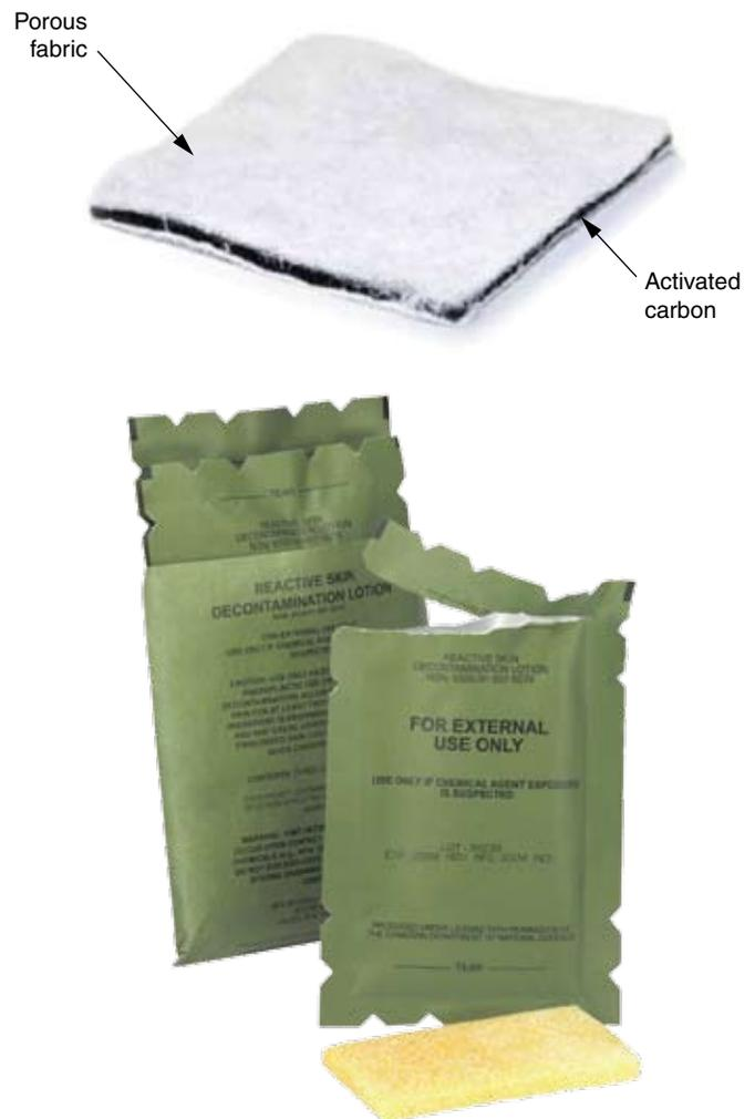
The low-cost personal decontamination system (LPDS) is an easy-to-use prototype kit for treating people or equipment after a chemical attack. A dry wipe (top image) removes the bulk of chemicals from the contaminated surface of skin or equipment. The yellow sponge is saturated with Reactive Skin Decontamination Lotion® to neutralize any residual chemicals.
